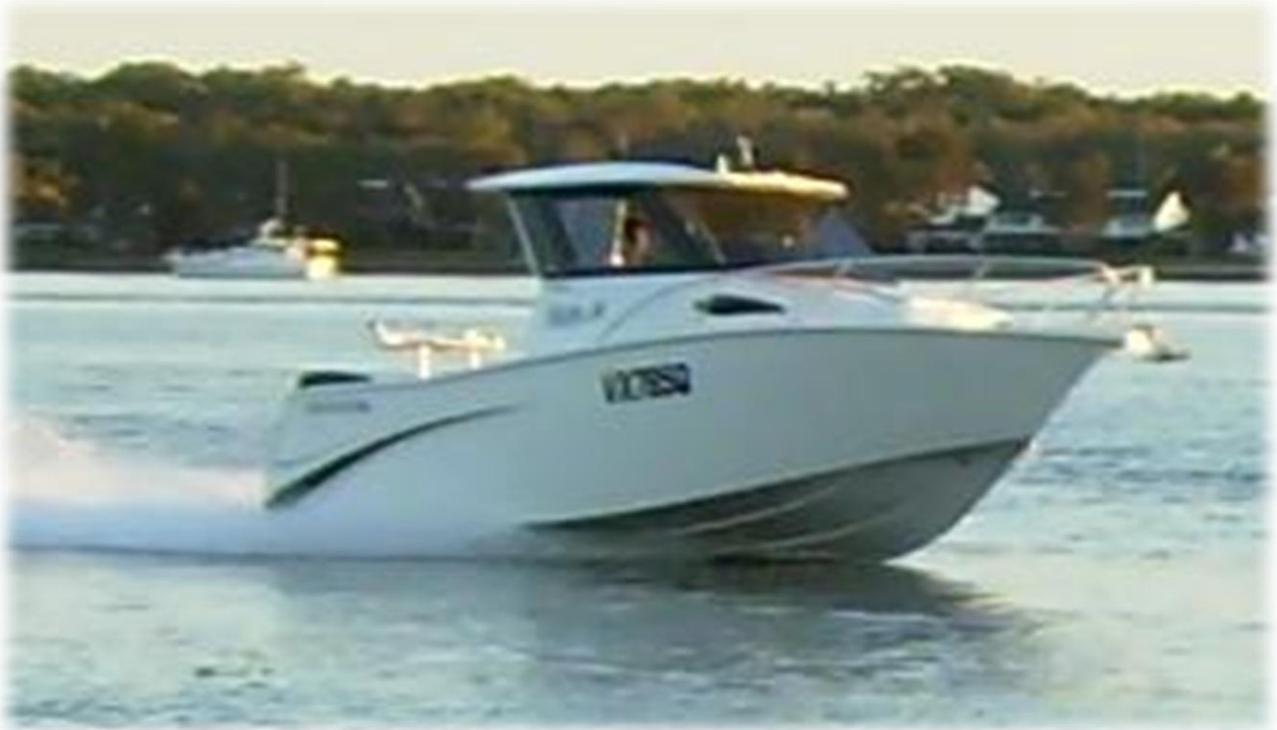
A confident stable hull designed for use both inshore and offshore conditions with good sea keeping capability. Offering a moderate 18-20 degree dead rise, fine entry bow and convex entry and planing surfaces this hull allows you to configure the topsides to suit your needs. From sport fisher to family day boat, it is only limited to your imagination.
